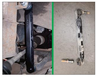
The wear in the ball joint allowed the arm to drop off on the journey to the garage, silencing the knocking noise
