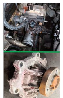
It was the thermostat housing leak that was spotted first, but the water pump had also been leaking and asked if he could have both jobs done at the same time, possibly cutting the cost a little.
