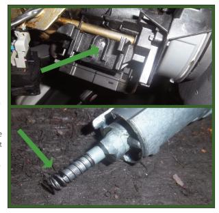
The end of the ignition barrel had broken meaning it was not making contact with the switch
