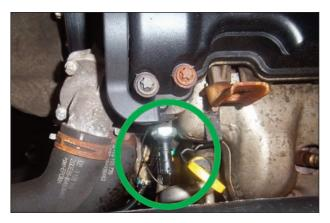
The source of the oil leak was spotted as soon as I looked under the bonnet and the oil pressure switch was easily replaced
