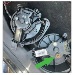
The corrosion on the old motor was a sign that water had entered the motor and caused its demise
