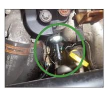
With the oil pressure switch replaced, the leak was halted.
