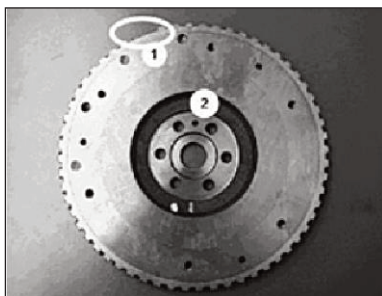
Flywheel teeth in the wrong position
