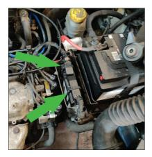
Cable ties had been used to secure the plugs
