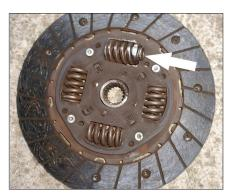
One of the centre plate springs had broke loose and was interfering with the clutch
