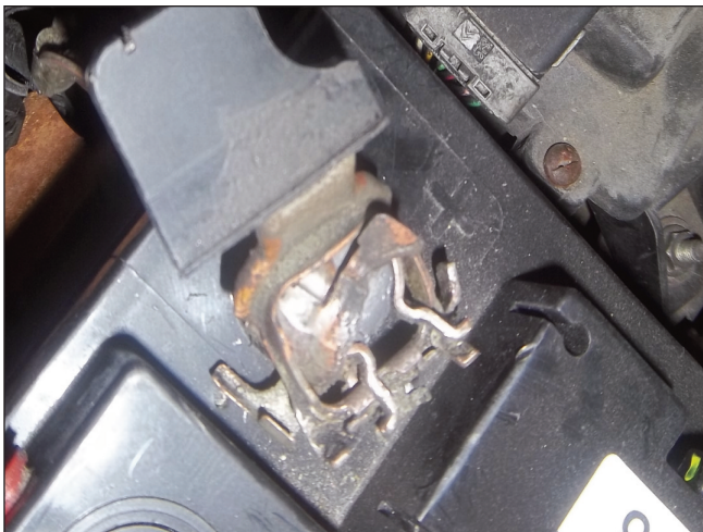
The battery terminal was the cause of all the problems
