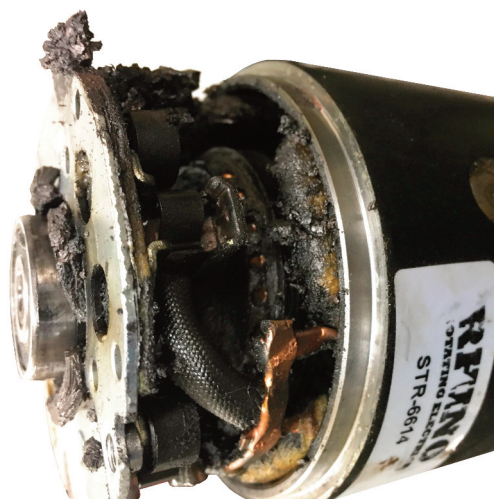
Diesel contamination had caused this Pajero starter to fail
