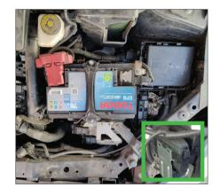
The fan relay is hidden under the left hand front headlamp and cannot be seen from above
