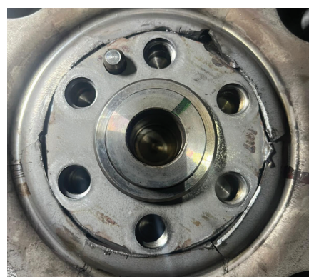
Logic showed the Cam signal was at least 100 degrees off, the result of the reluctor breaking and rotating to cause this unusual fault.
