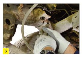
**Step 3** Tighten the coil firmly to the Mini-Ductor. **Step 4** Only heat the nut enough to expand and loosen. Red hot is too hot!
