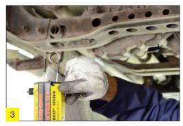
**Step 1** Make sure fuel lines are not leaking or creating a vapour
