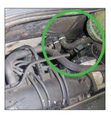
The telltale sign that a small jet of coolant had been spraying from one of the heater hoses
