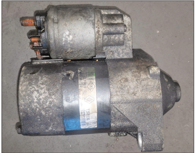
The old starter was displaying the Renault Logo and so was very likely the original unit
