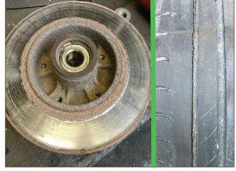
The vibration was the result of the poor condition of the tyres and the brake discs
