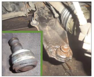
The lower swivel can be pressed out of the lower arm and the new one fitted without the need to remove the complete arm
