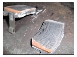
White patches on the brake pads are a sure sign of overheating and that the pads need to be changed
