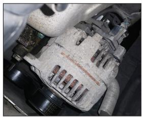
The alternator on the Seat Arosa is nicely accessible which makes the replacement job easy
