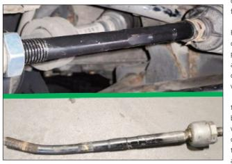
The impact had been absorbed by the track control arm which had bent and now required replacing
