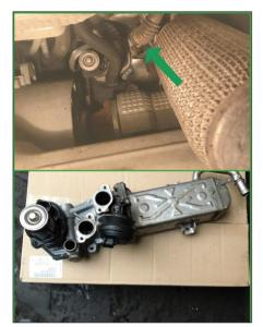
The unit with the cooler attached needs to be carefully manoeuvred out of position and the flexible pipes should be checked.
