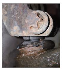
The perished rubber boot had allowed the dirt and grime from the road to enter the ball joint causing it to wear
