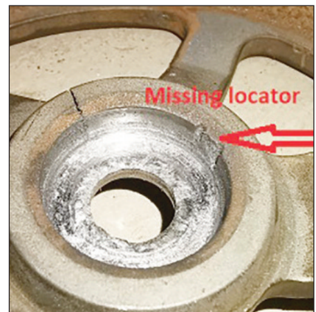
The pulley had been allowed to rotate on the camshaft after the locator sheared off
