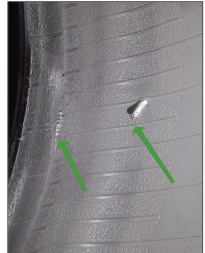
The screw had not only punctured the edge of the tread but also damaged the sidewall internally
