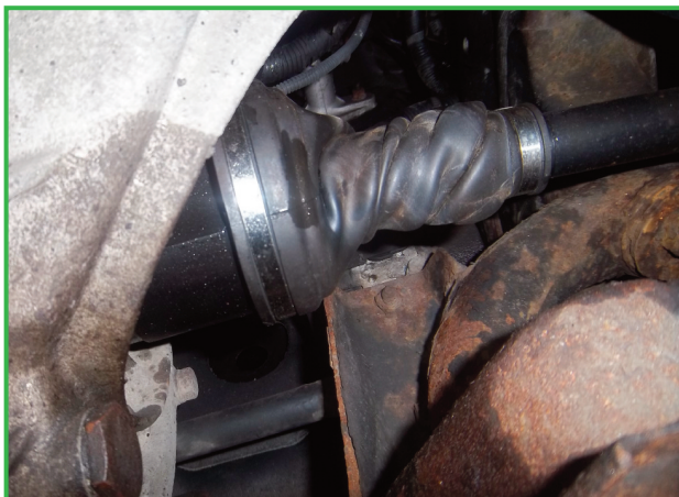
The new shaft had failed at the inner joint, spinning the boot up
