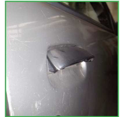
Staying in the up position when opening the door prevented the catch from operating correctly
