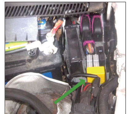
With the top housing cover removed the flasher unit is easily accessed and replaced
