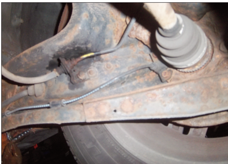
The corroded brake pipes were firmly rusted into the hoses, replacing these as well was the best option
