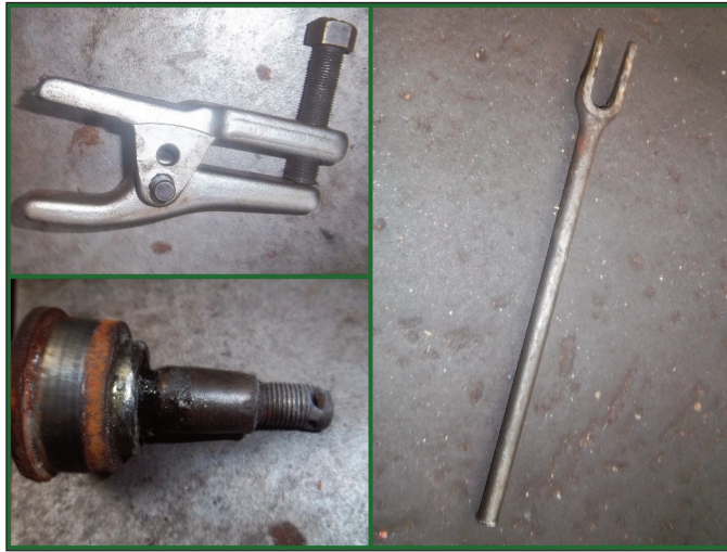
The swivel was squashed by the ball joint splitter; it may have been best to just use the fork type
