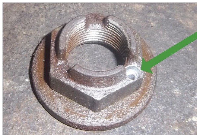
Drilling the hole in the nut released the pressure sufficiently to allow it to be removed
