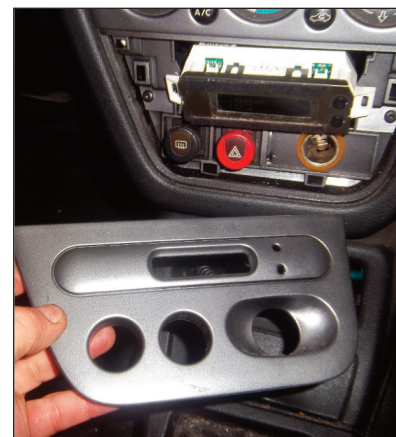
The front trim needs to be removed before accessing the screws securing the clock
