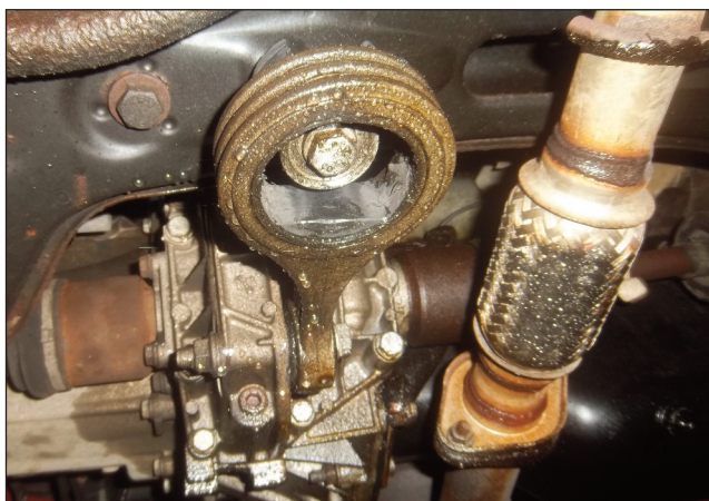
The centre bush had dropped from the tie bar allowing it to fall away from the fixing
