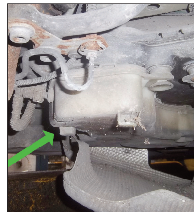
The Eolys fluid tank sits below the diesel tank
