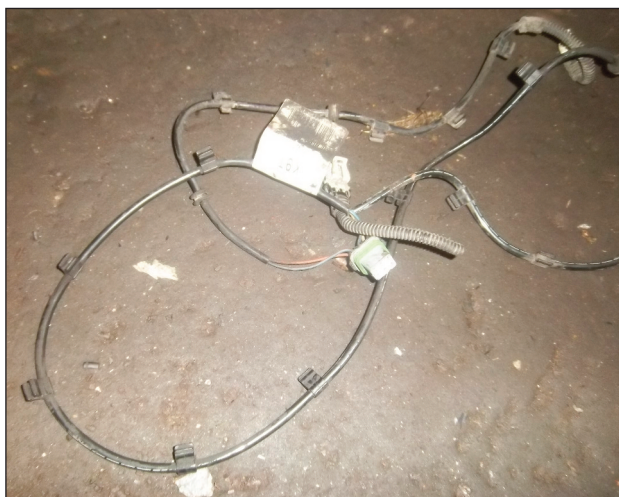
The wiring loom turned out to be the problem with the ABS system
