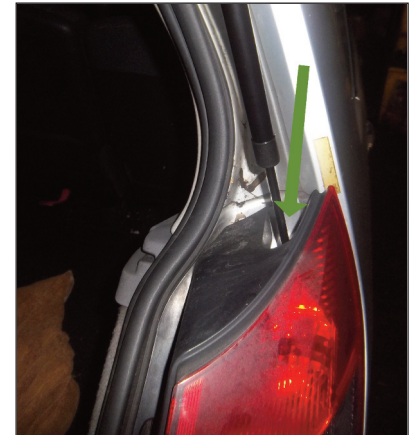
Before the struts could be changed the rear lamps had to be removed
