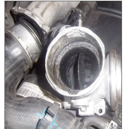
The EGR valve is regularly removed, cleaned and refitted, keeping it from blocking up with carbon deposits
