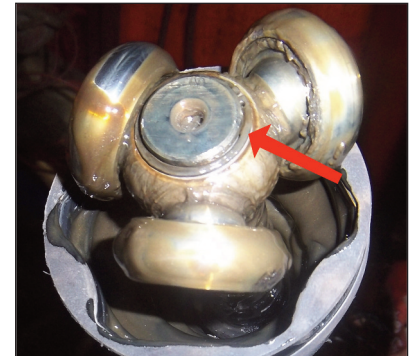
Once the circlip is removed the inner section of the joint will slide off the shaft
