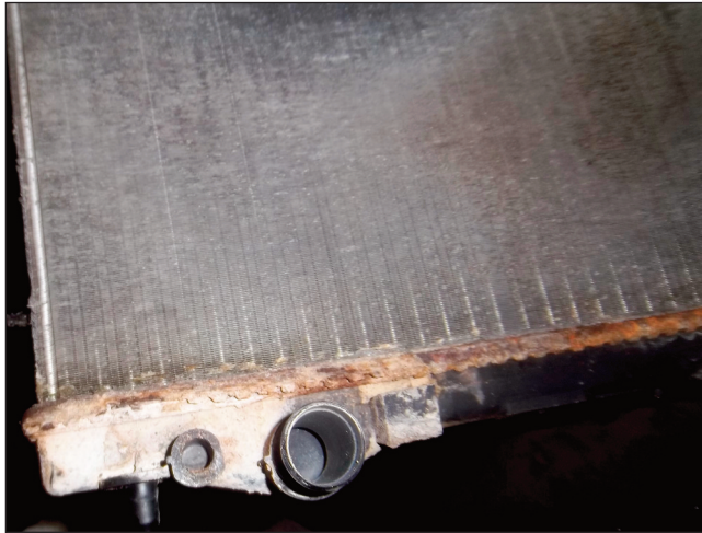
The radiator was rotten to the core, and even the best additive wasn't going to make it a serviceable unit
