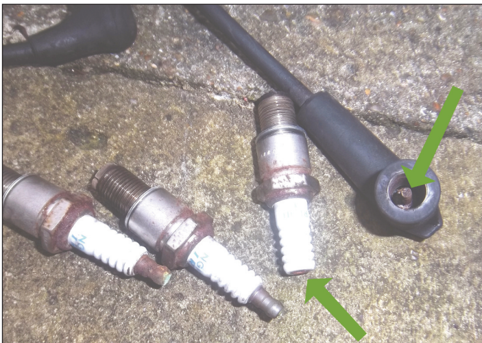
The Spark plug had a broken electrode which had remained attached to the removed HT lead
