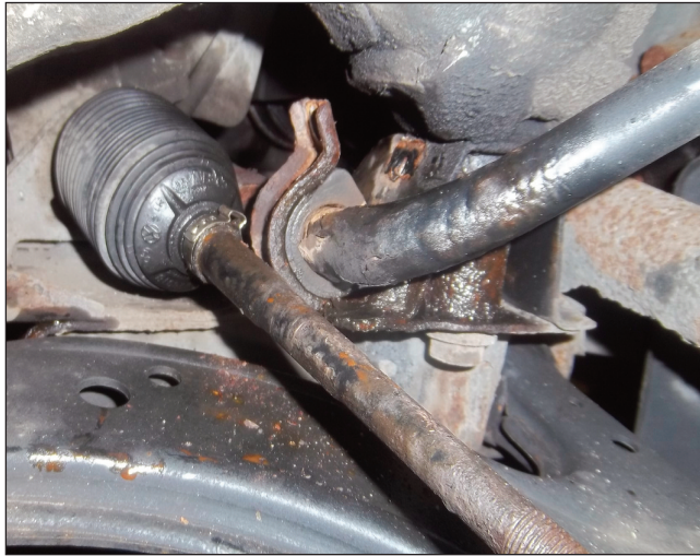
Removing the drop link, allows more movement and easier fitting of the new D bushes
