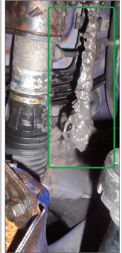
The plastic cover had not been successful at stemming the flow of leaking fluid
