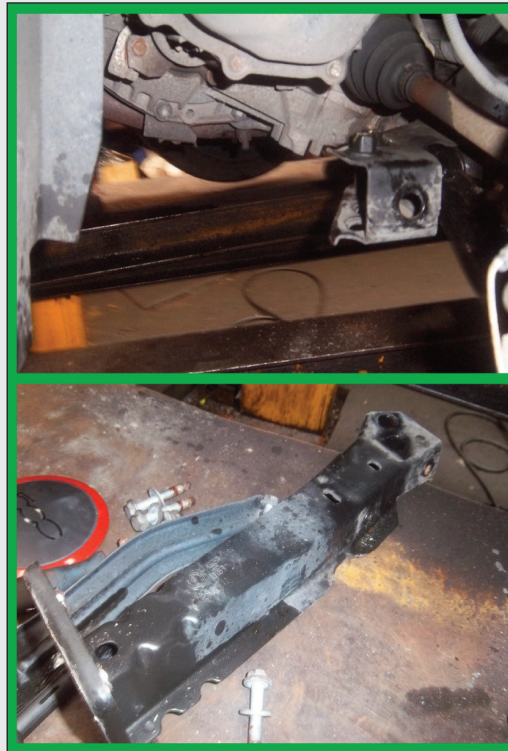
The box section needs to be removed before the arm securing bolt can be accessed
