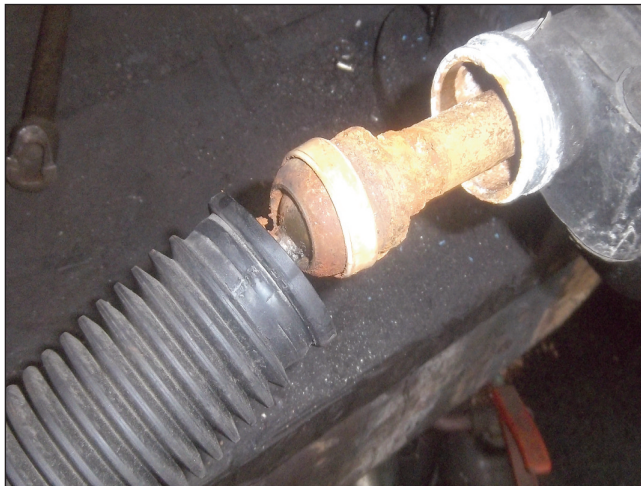
The steering rack had excessive rust in the unit cause by a lack of lubrication following a boot replacement
