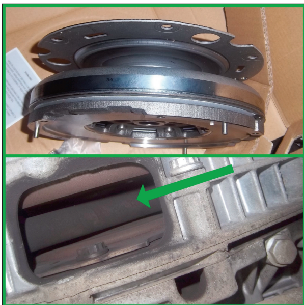
The drive shaft runs through the specially designed DMF unit
