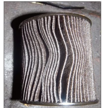
The oil filter was well past its best and was collapsing due to blockage and age
