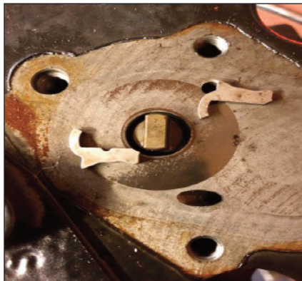
The pump had seized and snapped the drive mechanism
