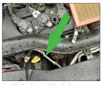
A soldering iron and insulating tape repair to the wiring saved the sensor from being replaced
