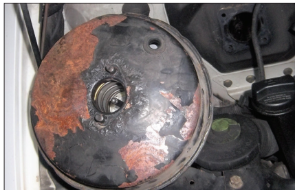
A failing servo unit was binding the brakes
