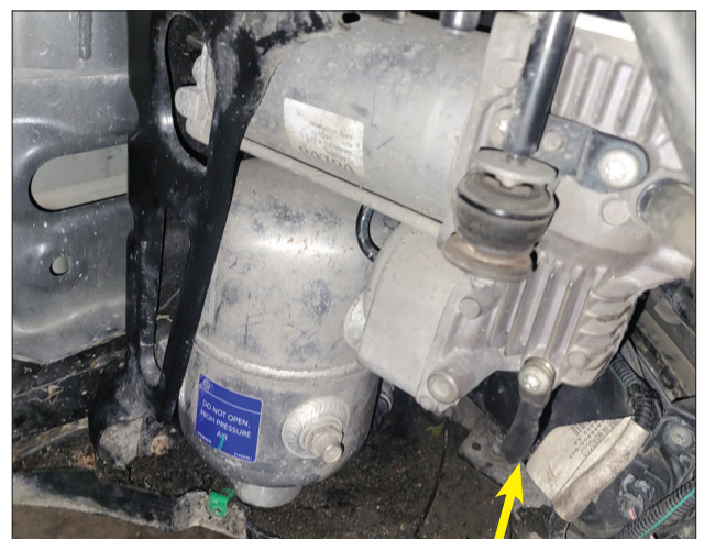
The PowerPulse temperature sensor (at arrow) looked more like an earth cable connection point
