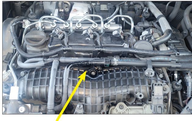
Oil residue (at arrow) indicated leak on inlet manifold
