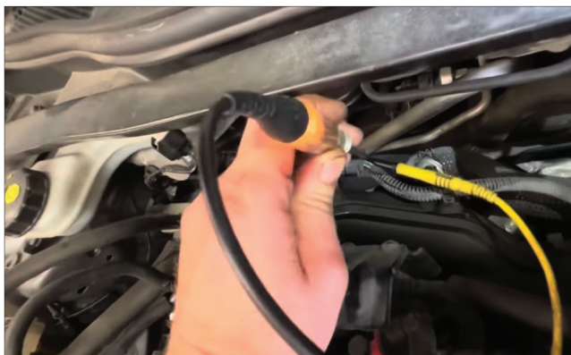
Use a 12V test light to load a circuit when you are testing the voltage on that circuit
