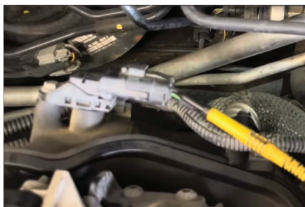
Voltage was measured by back probing each wire at the connector
