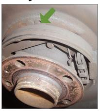
The retaining clips had broken away, allowing the shoes to fall out of place and rub the inside of the drum
