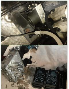
The ABS unit is fitted beneath the battery tray; the repair unit comes without the electronics which need to be fitted on
