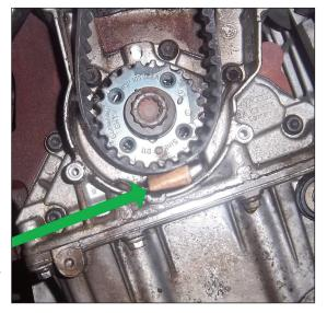
The small piece of cardboard is all that is needed to keep the belt in position whilst fitting
