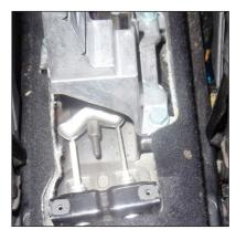
With new cables fitted the handbrake was smoother and the owner could now operate it without trouble
