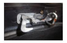
s part of our service, the secondary bonnet catch is always checked to ensure that it is free to move, will spring back into position after opening and will engage properly on closing. The importance of this catch operating correctly cannot be over emphasised.
