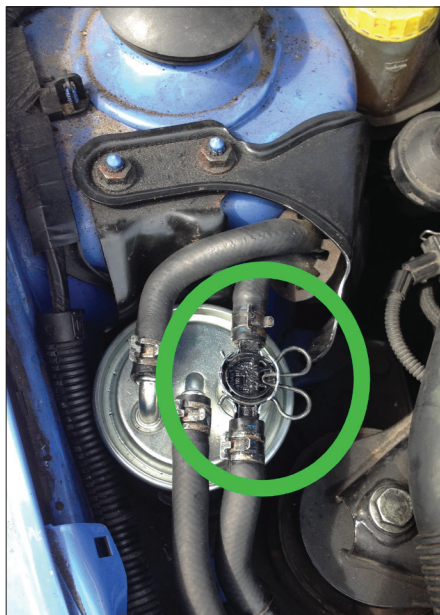
A weeping fuel filter seal was at the heart of the starting problems
