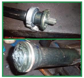
With the prop-shaft separated the centre bearing can be replaced
