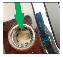
Debris in the exposed socket caused the unit to short out
