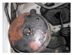
The cause of the overheating and brake binding problems was a failing servo unit something which can be overlooked
